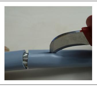
Remove the outer sheath to your required length using the stripping knife
