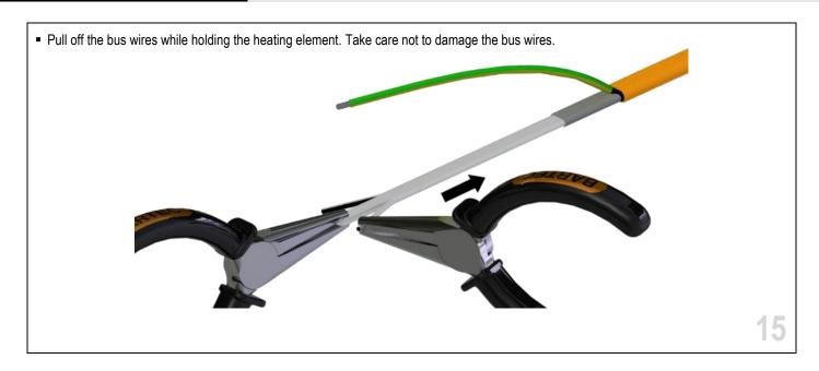
• Remove any remaining heating element that sticks to the bus wires.
