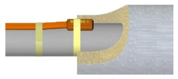
Recommendation for use of heating cable HSB+ and HTSB: install the end seal for protection of excessive heat above the insulation but below the outer cladding
