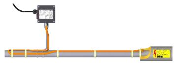
The trace heating system uses a self-regulating trace heater. It features a temperature-dependent resistive heating element that regulates and limits the heat according to the ambient temperature. If the ambient temperature rises, the power output of the trace heater is reduced. This self-regulating property prevents overheating which would cause damage to the trace heater. Crossing or overlapping with other parts of the same trace heating system is also possible.
