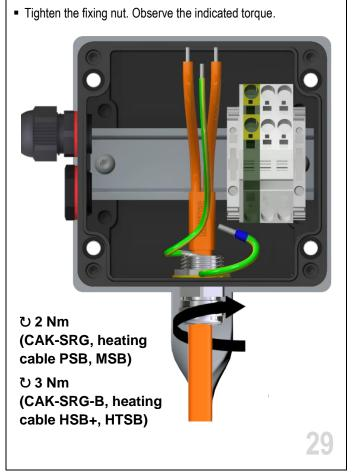
Slide the fixing nut onto the power cable.
